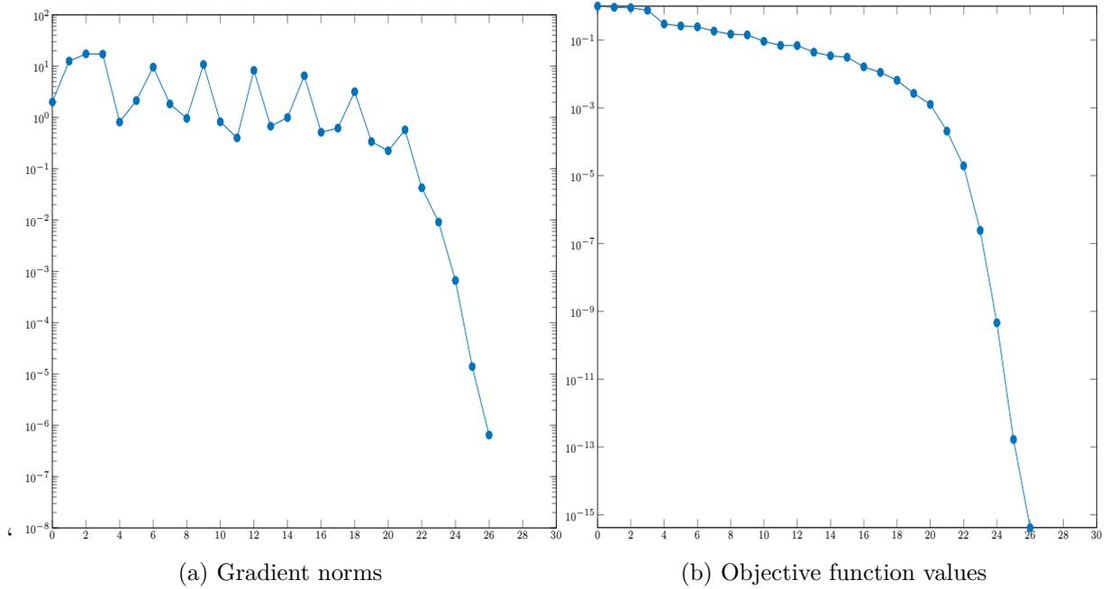
Figure 4: Gradient norms and objective function values (y-axes) w.r.t. iteration numbers (x-axis) for BFGS method (y-axis is log scaled, points at  $y = 0$  not shown due to log scale)
