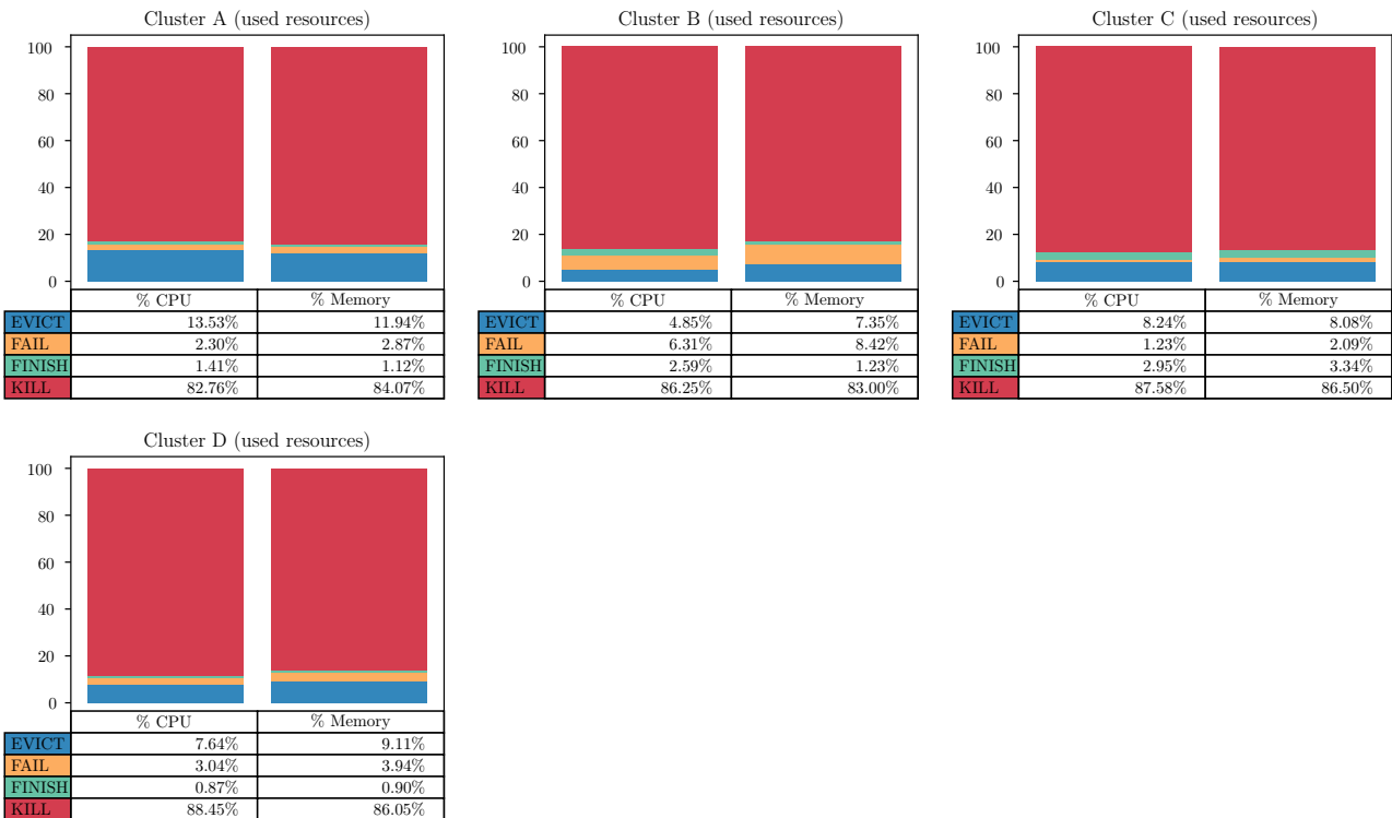
Figure 10. Percentages of CPU and RAM resources used by tasks w.r.t. task termination type for clusters A to D in 2019 traces. Refer to figure 9 for plot explanation.
