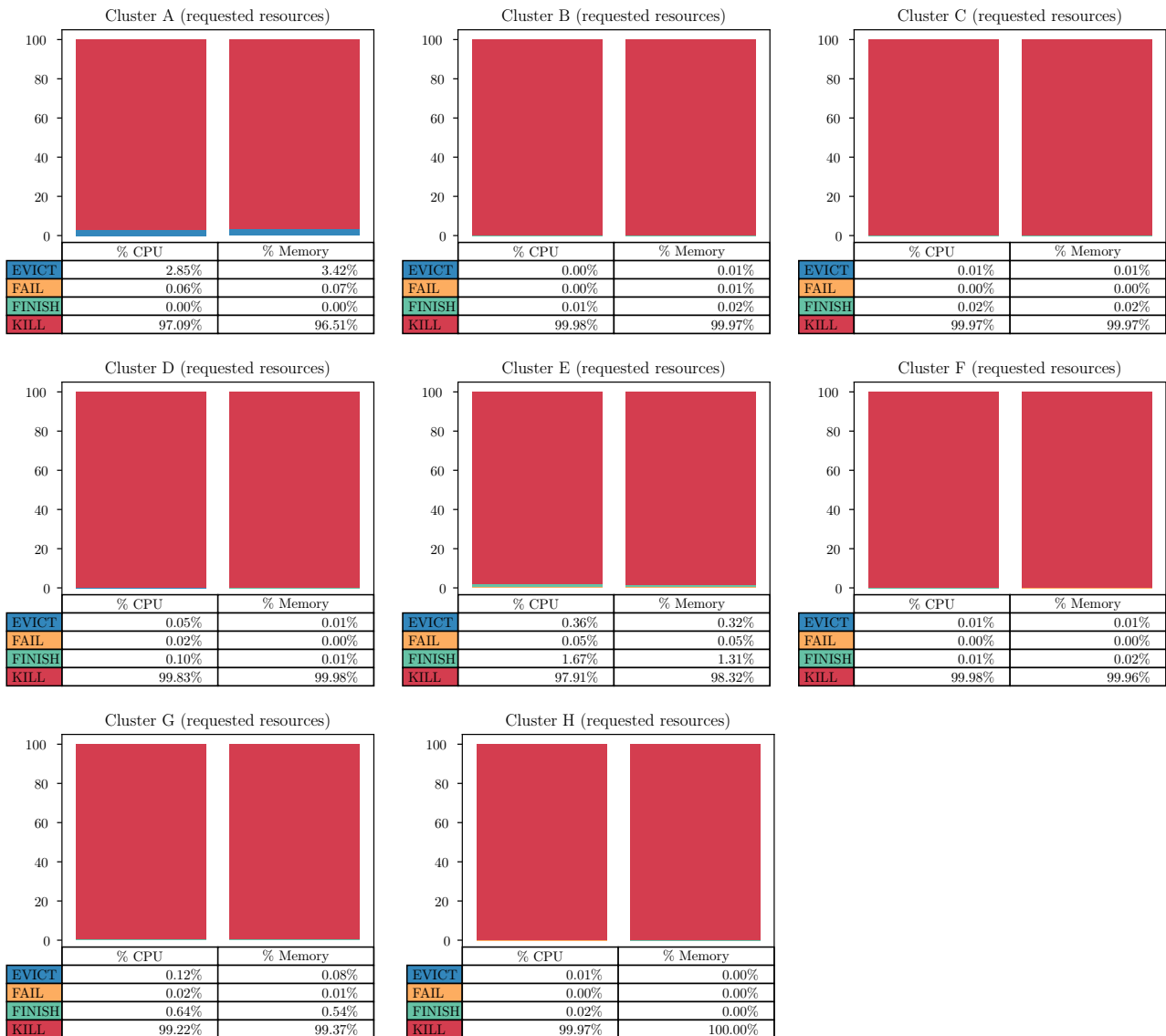
Figure 14. Percentages of CPU and RAM resources requested by tasks w.r.t. task termination type for in 2019 traces. Refer to figure 13 for plot explanation.
