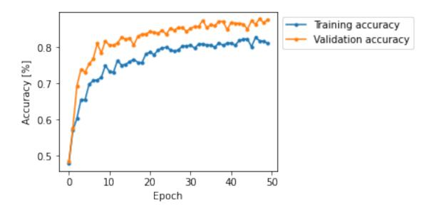
Figure 3: Training and validation accuracy curves during fitting for the data augmented VGG16 classifier
