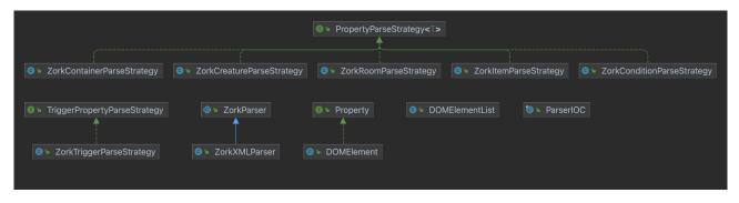
Figure 3: UML class diagram of the *com.github.dtschust.zork.parser* package
